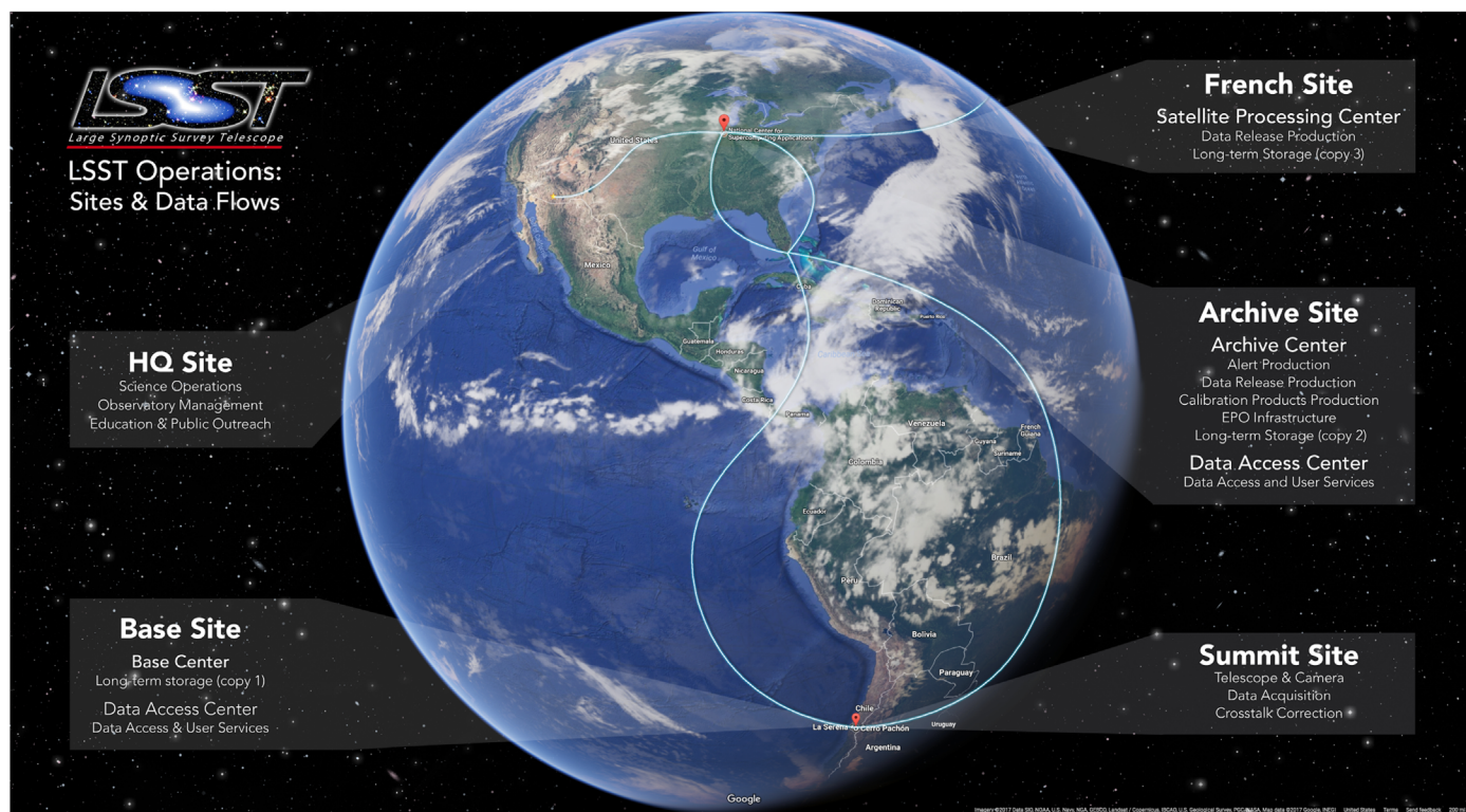
Figure 14. LSST data flow from the mountain facilities in Chile to the data access center and processing center in the US and the satellite processing center in France.
