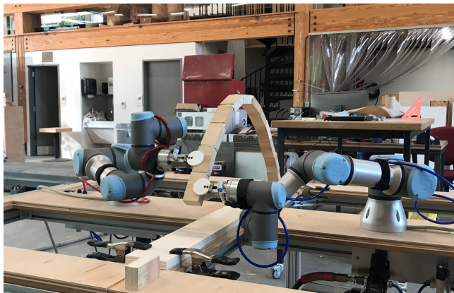
Figure 9: Small-scale prototype to test the alternating placement strategy for a brick arch with a running bond pattern
