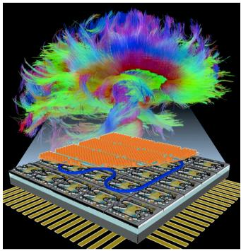
Figure 1. A conceptual rendering of a lightwave neuromorphic processor. Laser neuron arrays implement spiking dynamics with electo-optic physics, and a photonic network on-chip can support complex structures of virtual interconnection amongst these elements. Note: the colorful mind mapping (picture above the processor) was provided by the The Human Connectome Project.
