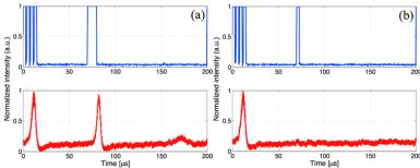
Figure 4. Experimental data of excitable fiber laser. (a) Traces showing a response to multiple integrated stimuli or one strong stimulus. (b) For too weak of an input, no change in output is detectable.
