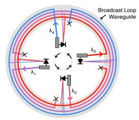
Figure 8. Conceptual diagram of a broadcast loop. The loop waveguide carries WDM channels from all participating PNNs. Each PNN detects a linear subset of the present channels. The PNN laser then outputs its signal, a function of those inputs, on its unique wavelength channel. Once a signal transverses the BL, it is terminated by its originating unit to avoid further interference. Filter banks and inhibitory pathways not shown.
