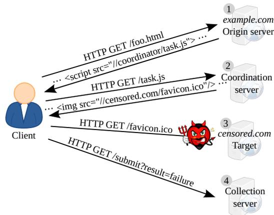
**Figure 2:** An example of observing Web filtering with Encore. The origin Web page includes Encore’s measurement script, which the coordinator decides should test filtering of `censored.com` by attempting to fetch an image. The request for this image fails so the client notifies the collection server.
