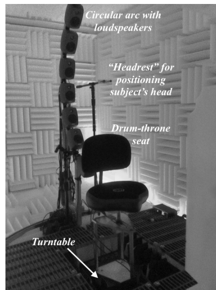
Fig. 1: Setup used to make HRTF measurements.
