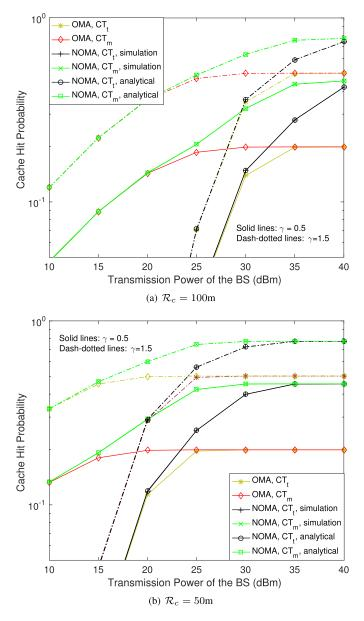
Fig. 6. The cache hit probability for the push-then-deliver strategy. N = 20,  $\alpha = 3$ ,  $\lambda_c = \frac{0.01}{\pi \mathcal{R}_c^2}$ , t = 5, m = 1,  $M_s = 3$ , and  $R_l = 1$  bit per channel use (BPCU), for  $1 \le l \le 3$ . The power allocation coefficient for file  $f_1$  is based on the CR power allocation policy. The power allocation coefficients for files  $f_2$  and  $f_3$  are  $\beta_2 = \frac{3}{4}$  and  $\beta_3 = \frac{1}{4}$ , respectively.  $|\mathcal{F}| = 10$ .
