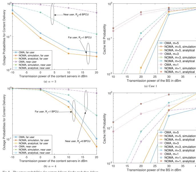
Fig. 8. The outage probabilities for content delivery for the push-then-deliver strategy. N = 20,  $\alpha = 4$ ,  $\mathcal{R}_c = 100$ m.  $\lambda_c = \frac{0.01}{\pi \mathcal{R}_c^2}$ ,  $R_1 = 1$  BPCU, and  $R_2 = 6$  BPCU. The power allocation coefficients are  $\alpha_1^2 = \frac{3}{4}$  and  $\alpha_2^2 = \frac{1}{4}$ .
