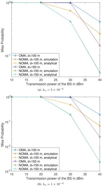
Fig. 11. The impact of the proposed push-and-deliver strategy on the cache miss probability in D2D caching scenarios. N = 20,  $\alpha = 3$ ,  $y_0 = (500 \text{ m}, 500 \text{ m})$ ,  $R_0 = 0.5 \text{ BPCU}$ ,  $R_1 = 4 \text{ BPCU}$  and  $M_s = 1$ . The power allocation coefficients are  $\alpha_0^2 = \frac{3}{4}$  and  $\alpha_1^2 = \frac{1}{4}$ .
