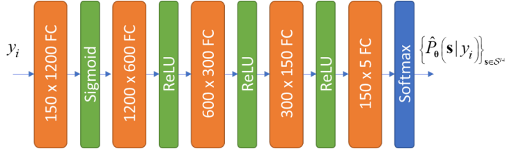
Fig. 4: The 5 FC network used for learning the function nodes.
