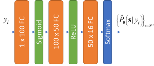
Fig. 7: The 3 FC network used for learning the function nodes.
