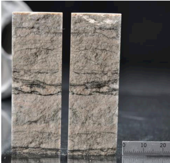
Figure 1. A photo of the fractured sub-core of Eau Claire formation.
