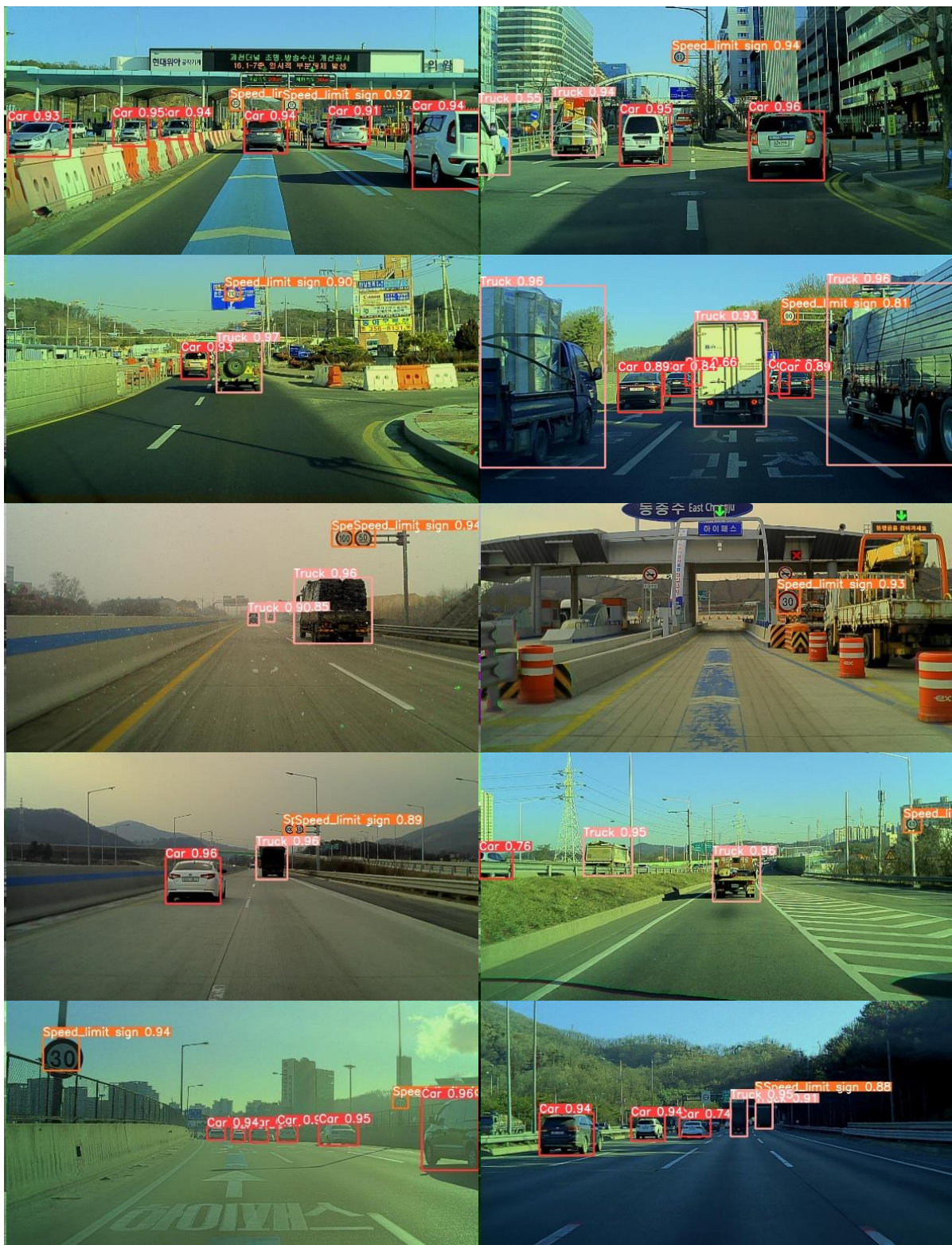
Figure 10. Various object detection results in different scenarios on K-roads.
