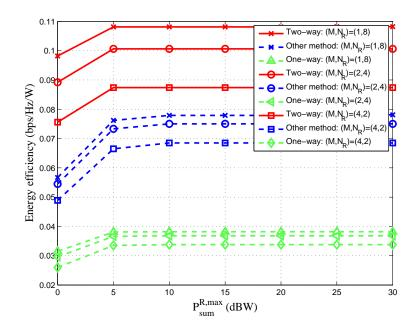
Fig. 8. Energy efficiency versus the relay power budget with K = 1
