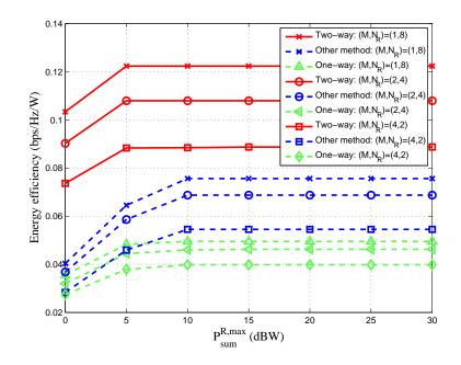
Fig. 5. Energy efficiency versus the relay power budget with K = 2
