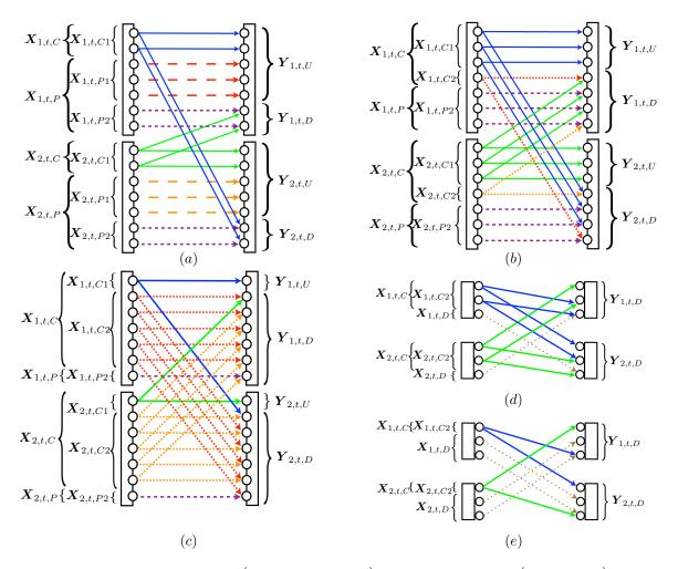
Fig. 6. Different components of channel input  $\mathbf{X}_{i,t} = (\mathbf{X}_{i,t,C}, \mathbf{X}_{i,t,P}, \mathbf{X}_{i,t,D})$  and channel output  $\mathbf{Y}_{i,t} = (\mathbf{Y}_{i,t,U}, \mathbf{Y}_{i,t,D})$  at channel use t, with  $t \in \{1, \dots, \max(N_1, N_2)\}$  and  $i \in \{1, 2\}$ , in the very weak interference regime (a), weak interference regime (b), moderate interference regime (c), strong interference regime (d) and very strong interference regime (e).
