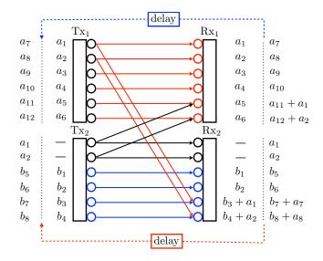
Fig. 4. Coding scheme for achieving the rate pair (6, 4) at an NE in the symmetric LD-IC with feedback, with n = 6 and m = 2.
