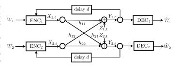
Fig. 1. Two-user Gaussian interference channel with perfect channel-output feedback at channel use t.
