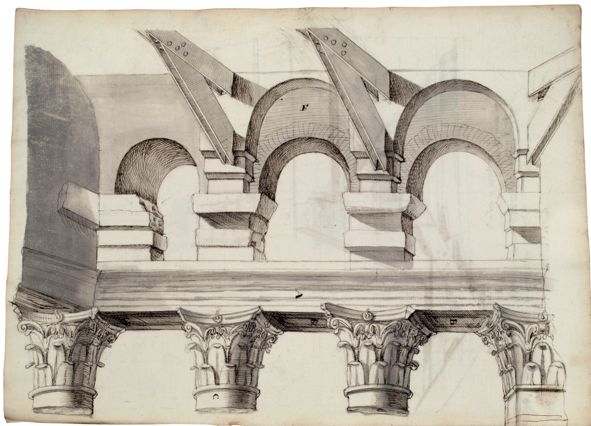
21. Anonymous 17th-century French draftsman. View of the roof structure of the Pantheon portico, ca. 1637–44. Pen and black ink with gray wash and graphite, 12 7 / 8 x 17 7 / 16 in. (32.7 x 44.3 cm). Worcester College Library, Oxford (MS B 2. 3, fol. 11v). Photograph: courtesy of the Provost and Fellows of Worcester College, Oxford
