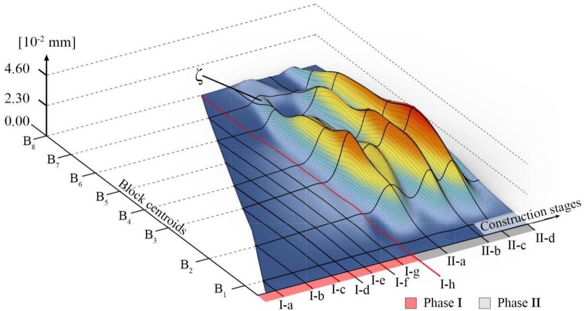
Figure 9. Displacement magnitudes surface ( $\zeta$ ). The vertical axis reports the magnitude of displacements. The other two axes represent the location of block centroids where the displacements have been recorded ( $B_1, B_2, B_3, \dots, B_8$ ) and the construction stages divided by the two phases **I** and **II**. Here, **I-a, I-b, I-c, \dots, I-h** are subdivisions in phase **I**, while **II-a, II-b** and **II-c** are the construction stage as described in figure 4.
