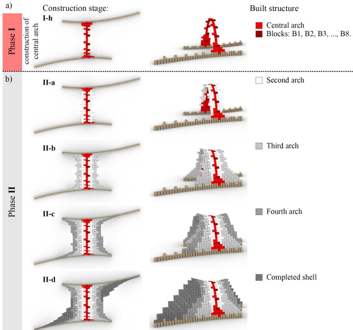
Figure 4. Construction process for the masonry vault.. a) Final stage of phase **I** and the closing of the central arch (construction stage **I-h**). b) phase **II**, where each stage is defined by the construction of a new inclined arch substructure.
